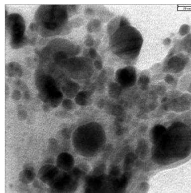
**Figure 1.** Transmission Electron Microscopy Image of Biosynthesized Silver Nanoparticles
