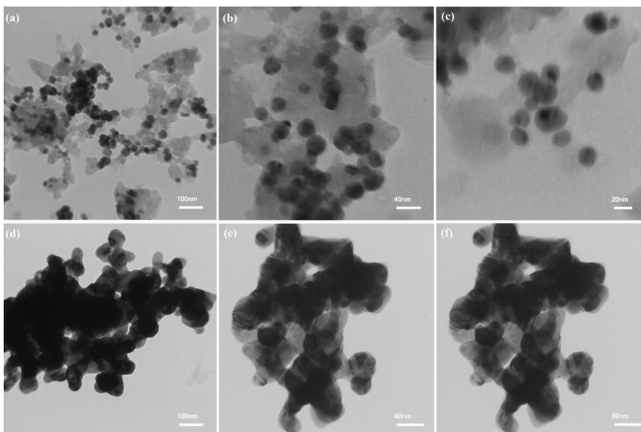
**Figure 3.** TEM Images (a-c) for the Green-Synthesized SNPs Prepared Using *E. thyrsoideum* and (d-f) Chemically Synthesized SNPs.
