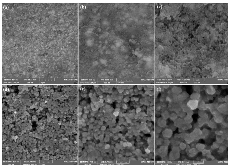
Figure 2. SEM Images (a-c) for Green-Synthesized SNPs Prepared Using *E. thyrsoideum* and (d-f) Chemically Synthesized SNPs
